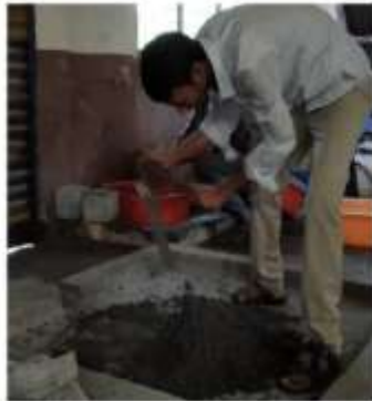
Figure 4.5 Casting of specimen
